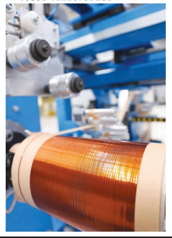
Windings are produced strictly matching with design parameters. Upon customer request electrolytic copper or aluminum is used as conductor, press band paper or kraft paper is used as insulator and proper wooden ducts are used for cooling. Materials are chosen as temperature resistant and cannot be dissolved in oil. Windings are manufactured in full automatic pc controlled machines.
